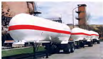
LPG Two & Three AXLE Semitrailers, Cap.: 9800 Gal.
